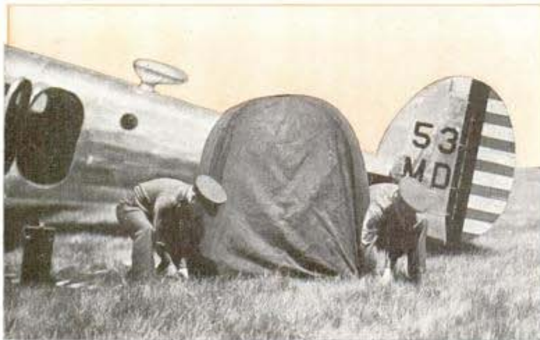
Four inflated pneumatic arches support this portable darkroom tent for developing film in the field. Black rubberized fabric makes it lightproof
